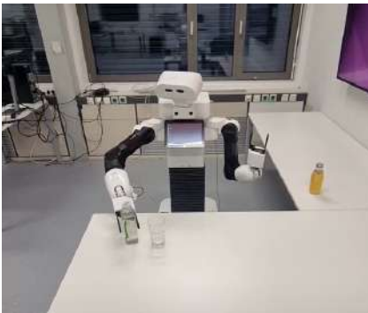
Figure 5.4. Bartending scenario with L-shaped table and dual-arm Tiago robot.
